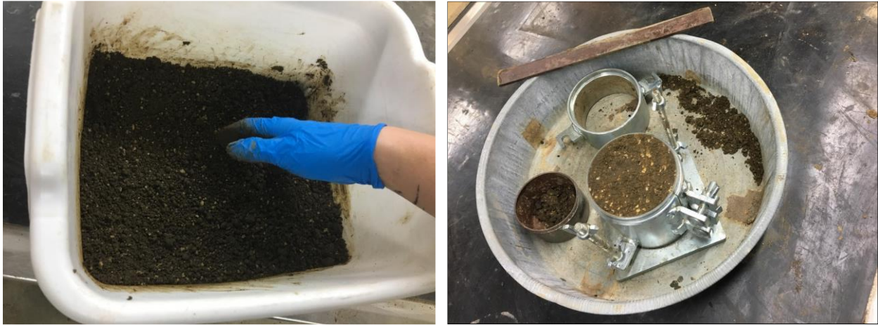
Figure 3.7 Proctor compaction test
