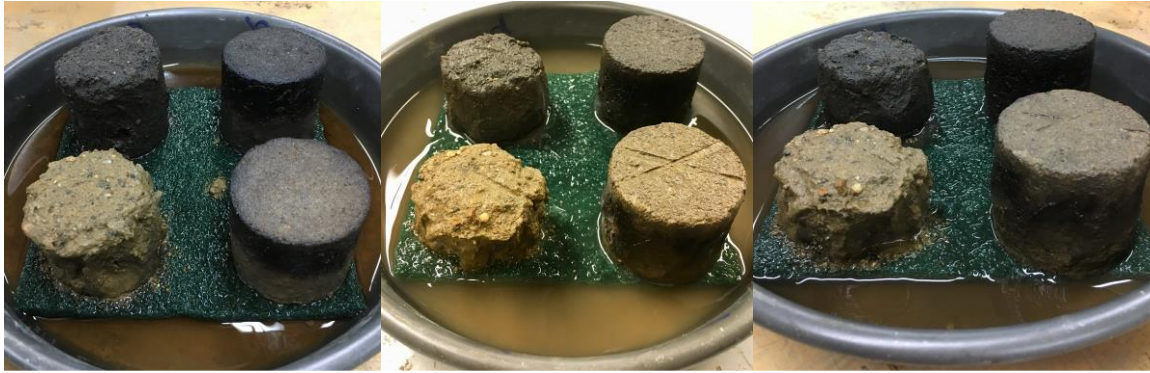
Figure 3.12 Specimens after 6 (left), 7 (middle), and 8 (right) cycles of freezing and thawing
